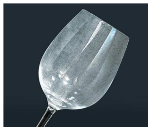
Hard water deposits
